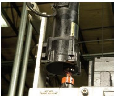
All motors are ball bearing type, rated for industrial duty. These motors, both AC and DC, are constructed from precision machined components and are dynamically balanced for smooth quiet operation.
