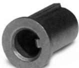
Reduces bore size of Quill type input shafts from 7/8 to 5/8. Sintered metal bushing with integral internal and external keys.
