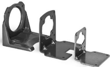
**Applications:** Mounting bracket for PSSH and PSL gearmotors. Securely mounts to gear face in 90 degree locations for floor, wall or ceiling mount. Catalog Number LB74 is not recommended for PSL/PSLH units weighing over 20 lbs. For units weighing more than 20 lbs. use Catalog Number LB75.
