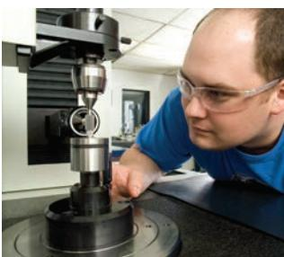
precision CNC machining centers and checked on state-of-the-art measuring equipment, these housing provide rigid support and accurate alignment of the gears.
